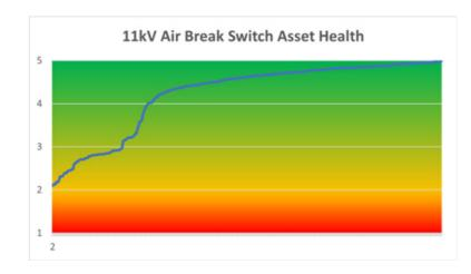
Figure 60 - Health Profile of Pole Mounted Air Break Switches
