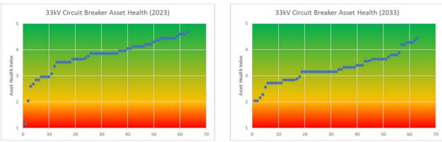
Figure 26 - 33 kV circuit breaker Asset Health 2023 (Current) and 2033 (Forecast)
