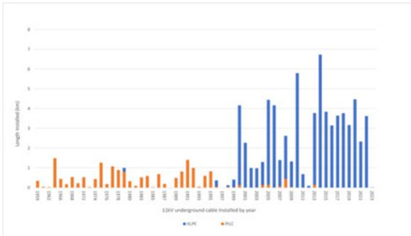
Figure 48 - Age profile of 11 kV cables
