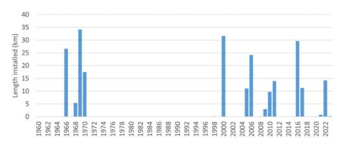
The health profile of these assets is shown below. Sub-transmission lines are often installed and replaced in large sections with the same material subject to similar environmental conditions. This is reflected in the "stepped" nature of the profile.
