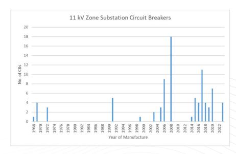
Figure 27 - 11 kV Zone Substation circuit breaker age profile
