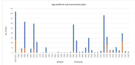
Figure 35 - Age profile for sub-transmission poles
