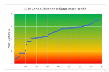
Figure 30 - Zone Substation Isolator Asset Health
