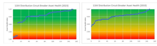
Figure 28 - 11 kV Distribution circuit breaker Asset Health 2023 (Current) and 2033 (Forecast)
