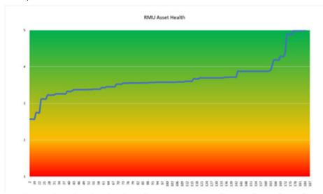
Figure 59 - Health profile of ground mounted distribution switchgear
