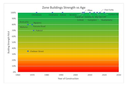
Figure 23 - Age and Strength profile for zone substation buildings
