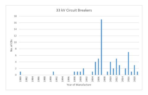
Figure 25 - 33 kV circuit breaker age profile
