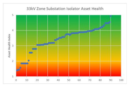
Figure 40 – Asset Health profile of sub-transmission Isolators
