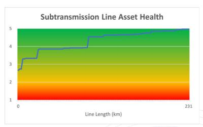
Figure 34 – Asset Health profile of sub-transmission overhead conductor
