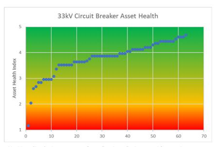
Figure 39 – Asset Health profile of sub-transmission Circuit Breakers , Reclosers and Sectionalisers
