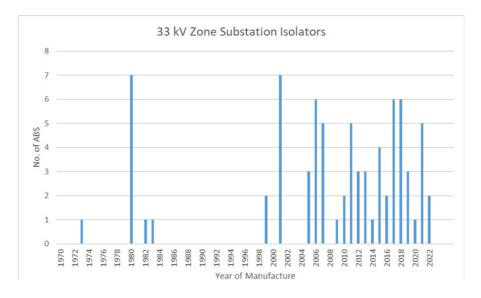
Figure 29 - Zone Substation Isolator Age Profile
