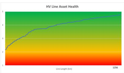
Figure 42 - Health profile of 11 kV overhead lines
